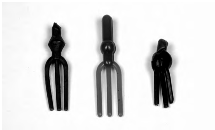
Figure 5.5 Special sprues for steam casting with balls on the sprue that function as risers
